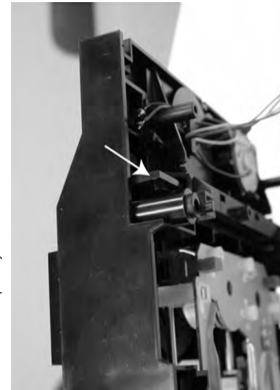
When a disc is loaded, unlock the tray by pushing the side inwards with a screwdriver and pull tray outwards.
